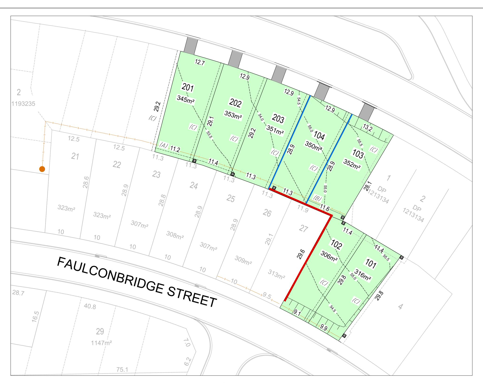
LEGEND DENOTES EASEMENT TO DRAIN WATER 1.0 WIDE. DENOTES EASEMENT TO DRAIN WATER 1.5m WIDE DENOTES EASEMENT FOR REPAIRS 0.9m WIDE DENOTES PROPOSED CONTOURS @ 0.5m INTERVALS **--**47.0·**-**-DENOTES 1V:6H BATTER (MAX. 4m LONG) DENOTES STORMWATER DRAINAGE DENOTES RETAINING WALL (MAX. 1.5m HIGH) DENOTES 1V:1H SIDE BOUNDARY BATTER FOR FUTURE DROP EDGE BEAM DENOTES CONCEPT SYDNEY WATER SEWER
